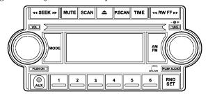
815eb156 REF Radio **NOTE:** The ignition switch must be in the ON or ACC position to operate the radio.
