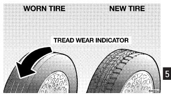
These indicators are molded into the bottom of the tread grooves. They will appear as bands when the tread depth becomes 1/16 inch (2 mm). When the tread is worn to the tread wear indicators, the tire should be replaced.
