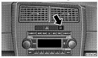
**NOTE:** To improve the vehicle's traction when driving with snow chains, or starting off in deep snow, sand, or gravel, switch off the TCS by pressing the TCS OFF button.
