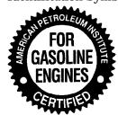
This symbol means that the oil has been certified by the American Petroleum Institute (API). The manufacture only recommends API Certified engine oils.
