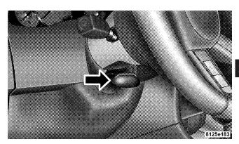
To unlock the steering column, pull the control handle outward. To tilt the steering column, move the steering wheel upward or downward as desired. To lengthen or shorten the steering column, pull the steering wheel outward or push it inward as desired. To lock the steering column in position, push the control handle inward until fully engaged.
