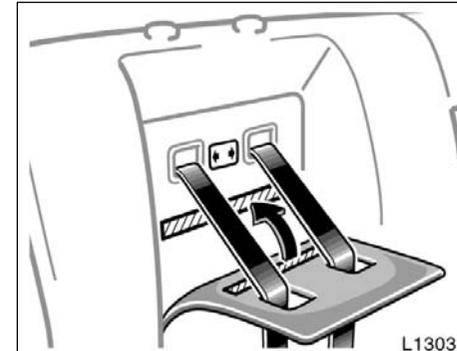
6. Press the removable pad against the fastener tapes and install the pad to the seatback. Make sure the belts go through the slots in the pad.
