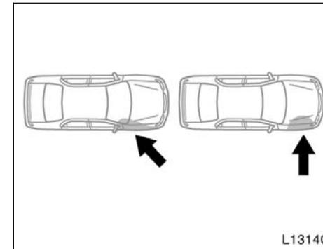
The SRS side airbags may not inflate if the vehicle is subjected to a collision from the side at an angle, or a collision to the side of the vehicle body other than the passenger compartment shown in the illustration, which impact is not severe enough for the passenger compartment.
