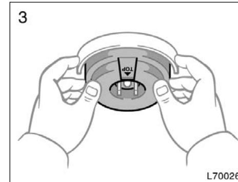
**3. Install the rubber cover with the "TOP" mark upward, and snugle on the boss. Insert the connector. Then install the plastic cover.**
