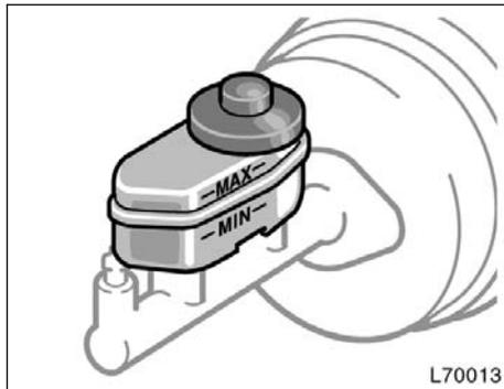
Use only newly opened brake fluid. Once opened, brake fluid absorbs moisture from the air, and excess moisture can cause a dangerous loss of braking.
