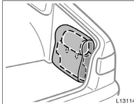
2. Insert the head restraint and upper pad into the storage bag. Then place the storage bag into the trunk by attaching with Velcro.
