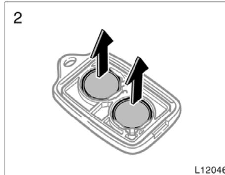
2. Remove the discharged transmitter batteries.
