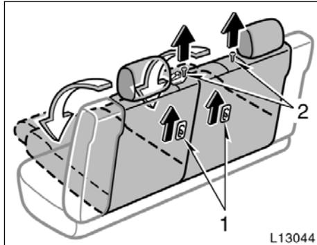
1. Pull up the seatback security lock lever 1 to the unlock position.
